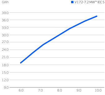
Assumptions One wind turbine, 100% availability, 0% losses, k factor = 2 Standard air density = 1.225, wind speed at hub height
